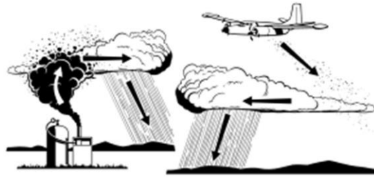
Fig.1. Cloud seeding can be done by ground generators, planes, or rockets
