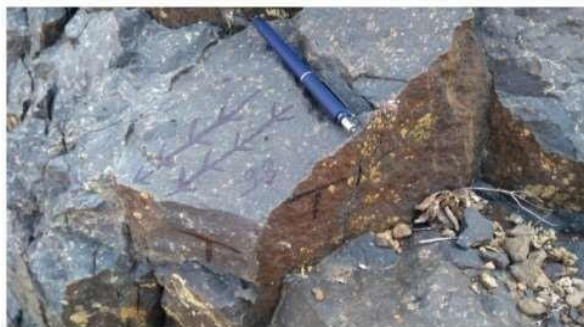
Fig. 3. An in-situ outcrop sample is oriented using a Brunton compass for the north marking arrow and a spirit level for horizontal marking.
