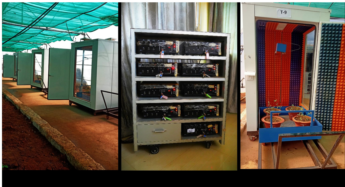
Fig. 1. Photographs of Acoustic Growth Chambers hosted in a polyhouse fitted with speakers and connected to a control panel to dispense musical treatment to plants.
